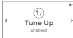
Enabling **Tune Up** helps you achieve a more stable tuning by having Roadie 4 first drop slightly below the target note, then tighten up to pitch. This ensures every string settles with tension pulling in the same direction, at the nut, saddle, and tuning post, reducing slippage and helping your guitar stay in tune longer.
