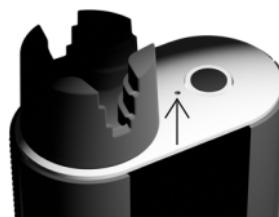
Insert a pin into the reset pinhole located between the power button and the tuning peg connector. You'll hear a click and the screen will turn off.
